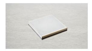
The multilayer piezo actuators can reach full performance at very low operating voltage. The plate actuator NAC2015 is 10x10 mm and provides a free stroke of 3.3  $\mu$ m and a blocking force of 4200 N.
