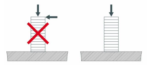
The actuators without preload are sensitive to pulling forces. It is recommended to apply a pre-load in order to optimize the performances of the actuators.
