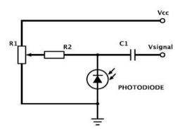
We recommend using **photovoltaic mode**, when PD is used under no reverse bias. Use photoconductive mode (mode with reverse bias) with caution.
