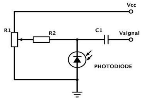
We recommend using **photovoltaic mode**, when PD is used under no reverse bias.
