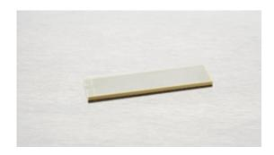
Noliac plate benders are manufactured with ceramic layer thickness down to  $67\mu m$  as standard to facilitate very low operating voltage for full performance of the piezo material. CMBP06 measures 32x7.8x1.8 mm. The plate bender provides stroke of +/-210  $\mu m$  and a blocking force of 4.3 N.
