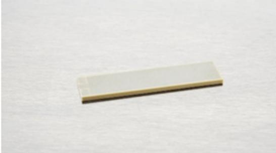
Noliac plate benders are manufactured with ceramic layer thickness down to 67µm as standard to facilitate very low operating voltage for full performance of the piezo material. CMBP04 measures 32x7.8x0.7 mm. The plate bender provides stroke of +/- 475 µm and a blocking force of 0.75 N.
