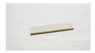
Noliac plate benders are manufactured with ceramic layer thickness down to  $67\mu m$  as standard to facilitate very low operating voltage for full performance of the piezo material. CMBP03 measures 21x7.8x1.8 mm. The plate bender provides stroke of +/-  $85~\mu m$  and a blocking force of 5.5~N.
