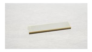
Noliac plate benders are manufactured with ceramic layer thickness down to  $67\mu m$  as standard to facilitate very low operating voltage for full performance of the piezo material. CMBP01 is currently the smallest standard plate bender from Noliac measuring 21x7.8x0.7 mm. The plate bender provides stroke of +/- 195  $\mu m$  and a blocking force of 1.2 N.
