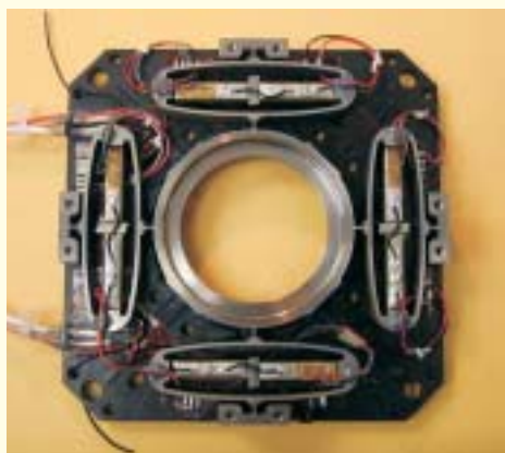
Figure 2: XY200M-SG space version stage with Strain Gages option - Opened top view.
