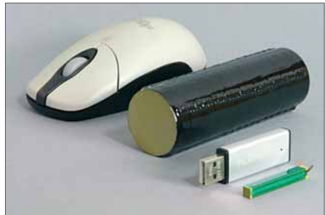
Fig. 2.1: High voltage stack (black, left) and low voltage stack (green, right), mouse and USB stick for size comparison.
