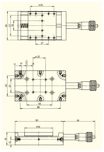
All threads M 4 All counterbores Inbus M 4 All dimensions in mm
