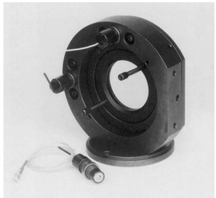
Fig. 4: 2-dim tilting mirror mount with FPSt screwed in piezocartridges for OptiSeek Control of a laser resonator
