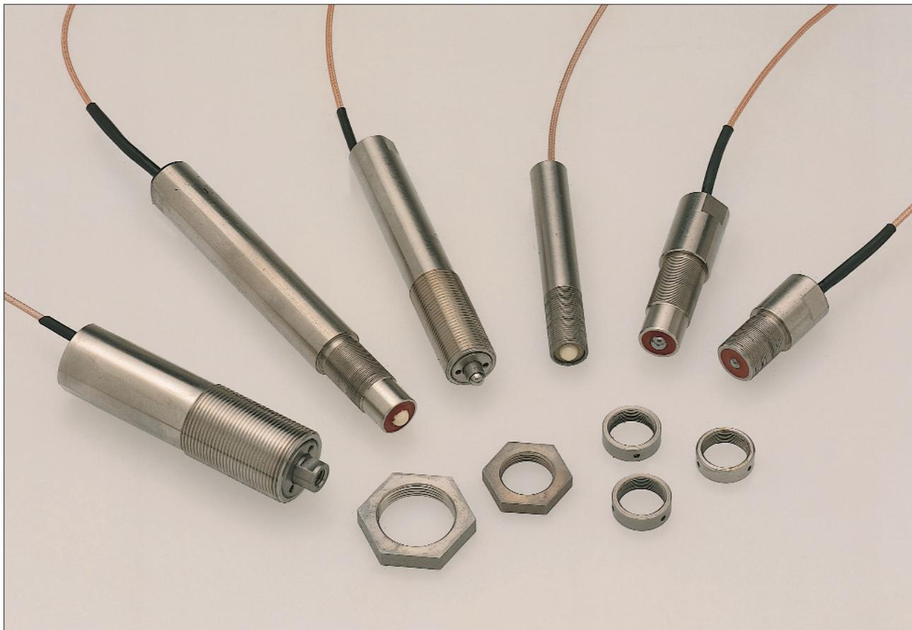
Stack actuators in cartridge-version offer elegant design features by simple attachment of an actuator to the mechanics using a front mounting thread. Using this thread a coarse adjustment for the system is provided. Piezocartridges can retrofit conventional lead screws. Mechanical arrangements for adjusting purposes can be very simply upgraded by using piezocartridges.
