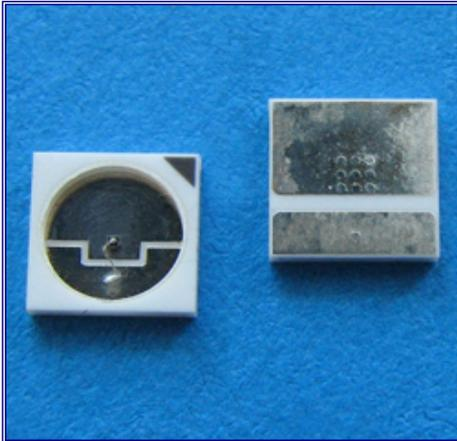
Light Emitting Diodes with central wavelength 4,15  $\mu\text{m}$  series are based on heterostructures grown on InAs substrates by MOCVD. InAsSb is used in the active layer. Wide band gap solid solutions InAsSbP with P content 50% are used for good electron confinement.
