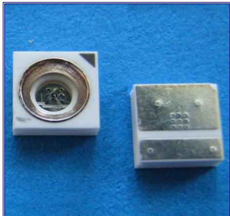
Light Emitting Diodes with central wavelength 3,55  $\mu\text{m}$  series are based on heterostructures grown on InAs substrates by MOCVD. InAsSb is used in the active layer. Wide band gap solid solutions InAsSbP with P content 50% are used for good electron confinement.
