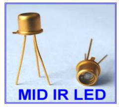
Light Emitting Diodes with central wavelength 3,40  $\mu m$  series are based on heterostructures grown on InAs substrates by MOCVD. InAs is used in the active layer. Wide band gap solid solutions InAsSbP with P content 50% are used for good electron confinement.
