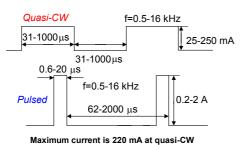
Maximum pulsed current is 1 A (duration 500 ns, repetition rate 2 kHz) Optimal operating current is 150-200 mA at quasi-CW.
