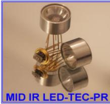
Light Emitting Diodes with central wavelength 2,84  $\mu m$  series are based on heterostructures grown on InAs substrates. InAsSbP is used in the active layer. Wide band gap solid solutions InAsSbP with P content 50% are used for good electron confinement.
