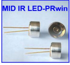
Light Emitting Diodes with central wavelength 2,84  $\mu m$  series are based on heterostructures grown on InAs substrates. InAsSbP is used in the active layer. Wide band gap solid solutions InAsSbP with P content 50% are used for good electron confinement.
