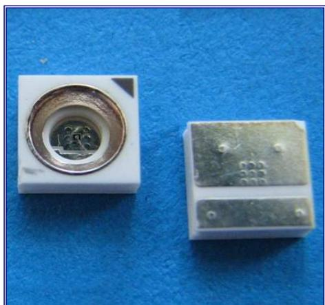
Light Emitting Diodes with central wavelength 2,05  $\mu\text{m}$  series are based on heterostructures grown on GaSb substrates by LPE. Solid solutions GaInAsSb are used in the active layer. Wide band gap solid solutions AlGaAsSb with Al content 64% are used for good electron confinement.
