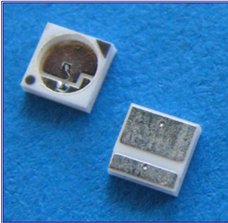
Light Emitting Diodes with central wavelength 2,05  $\mu\text{m}$  series are based on heterostructures grown on GaSb substrates by LPE. Solid solutions GaInAsSb are used in the active layer. Wide band gap solid solutions AlGaAsSb with Al content 64% are used for good electron confinement.
