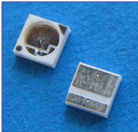
Light Emitting Diodes with central wavelength 1,88  $\mu\text{m}$  series are based on heterostructures grown on GaSb substrates by LPE. Solid solutions GaInAsSb are used in the active layer. Wide band gap solid solutions AlGaAsSb with Al content 64% are used for good electron confinement.
