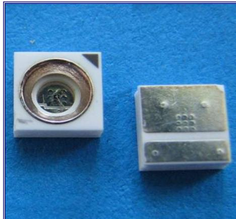
Light Emitting Diodes with central wavelength 1,85  $\mu\text{m}$  series are based on heterostructures grown on GaSb substrates by LPE. Solid solutions GaInAsSb are used in the active layer. Wide band gap solid solutions AlGaAsSb with Al content 64% are used for good electron confinement.
